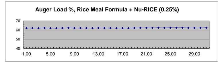
Summary:Rice was ground to a 30-40 screen size.<br/>Rice meal dry blended with the Nu-RICE, then hydrated to desired %.<br/>Nu-RICE was used to help the rice absorb the water, reducing the surface moisture & to improve hydration.<br/>Rice meal formulation + Nu-RICE ran much better than the control and product was on specification.
